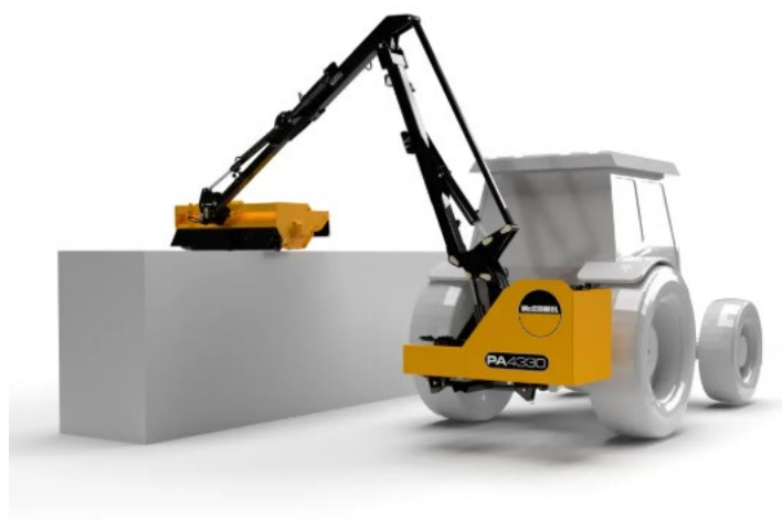
Figure 6 – Example of McConnell hedge flail with 4.5m reach
