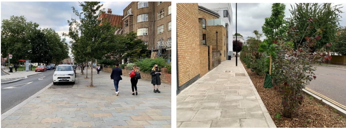
Figure 6-14: Example of a recessed loading/parking (Clapham Old Town, left) and example of clear footway space incorporating SuDS (Crossway, London, left)
