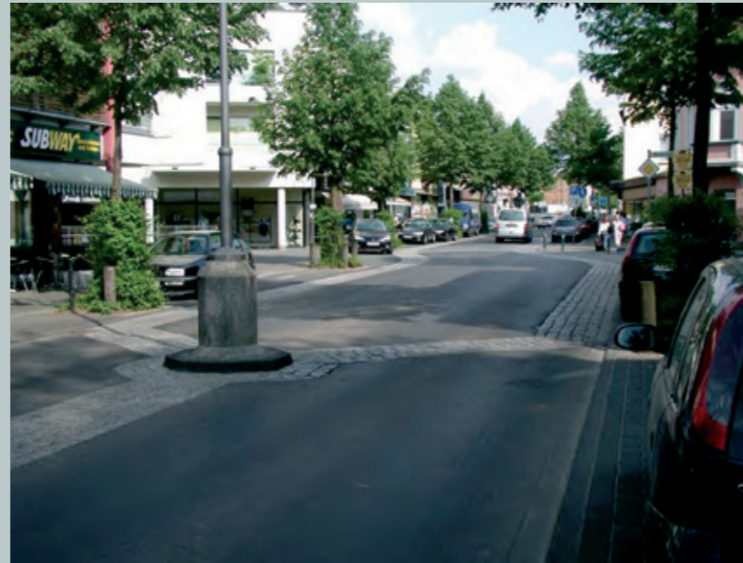
Street features in the centre, low kerbs and differently textured surfaces
